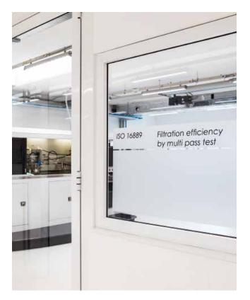
examination. The tests, carried out to verify the characteristics of the filters, are performed in accordance with international standards within controlled and filtered climate chambers, reproducing the operating conditions of pressure and flow rate of any hydraulic circuit.
